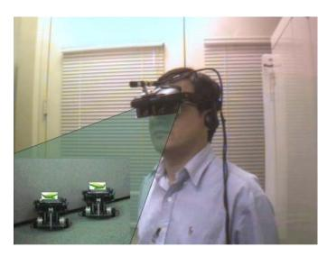
Figure 6: Coded infrared signals are decoded into arrows for overlay onto a real scene. These are visible via the augmented reality head-mounted display system with camera.
